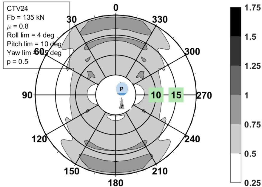
Finally, when the accessibility rose is known, computing the accessibility for the current sea state only implies considering the platform orientation and doing a simple 2D interpolation.
